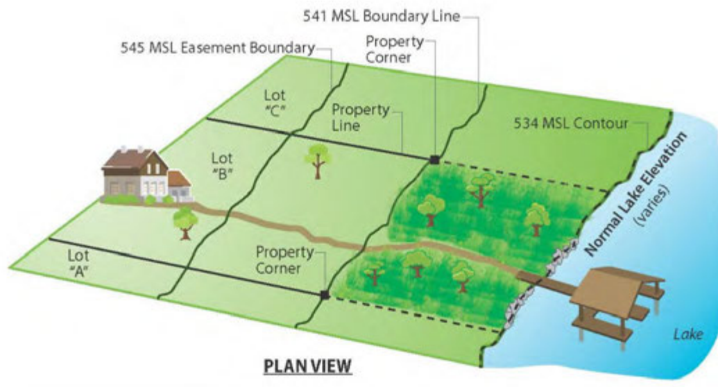
Figure 4-4. Property Boundary Equivalent and Hard Erosion Control BMP Installation
